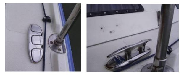
The through bolts for the cleats pass through the side deck. On the starboard side they emerge in forward locker; on the port side in the galley locker. Access for fitting is fairly easy, and I have backed them with 10mm marine ply pads epoxied to the under side of the deck.
