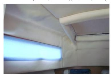
For that part lying under the mast, the lining was glued to a sheet of hardboard which was screwed in place – this allowed access to mast foot bolts. The rim of the hatch was covered using separate strips of headlining but using the overlap technique described earlier where there were butted joins.
