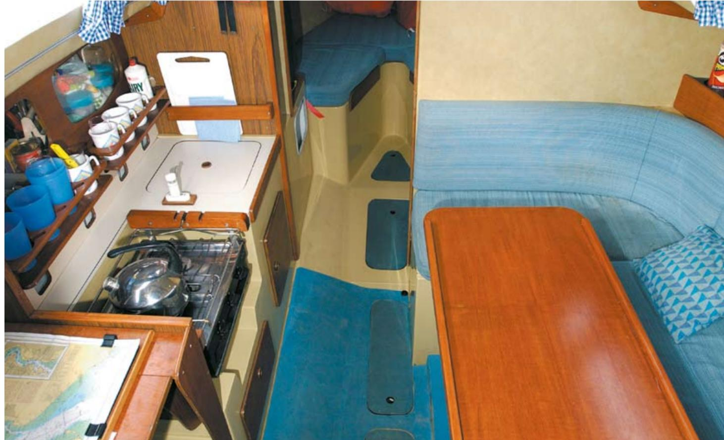
Below: *Incamoon* has a folding chart table at the head of the port quarter berth. A Yeoman plotter is mounted on a board that fits on top of the table and VHF and other instruments are mounted outboard for easy use
